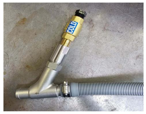
2. Remove black plug and attach cold water line. Drain Water Tempering assembly must be no higher than 12" from the floor.
