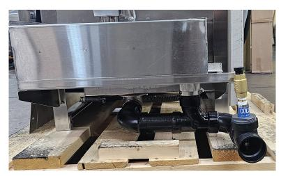
2. DWT with elbow installed before the tee with black plug installed.
