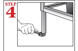
Level dishmachine by adjusting leveling legs. Dishmachine must be level front and back to ensure proper performance.
