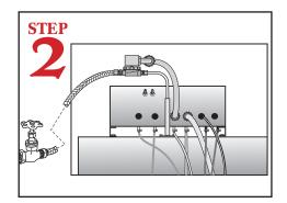
Connect dishmachine to hot water source (minimum 120-140 temperature required).
