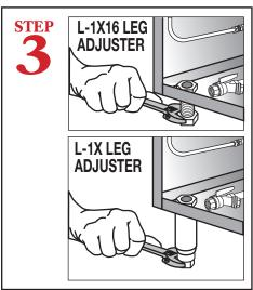
Level dishmachine by adjusting leveling legs. Dishmachine must be level front and back to ensure proper performance.
