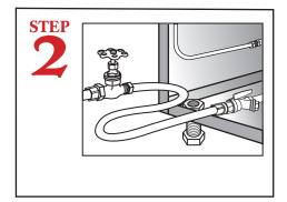
Connect dishmachine to hot water source recommended 140° temperature (120° minimum temperature required).
