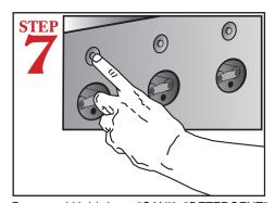
Press and Hold down "SANI", "DETERGENT" and "RINSE" switches to prime chemicals. This step must be repeated each time chemical containers are changed.
