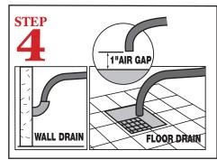
Connect the drain hose to wall or floor drain. The floor drain must have a 1 inch air gap between drain hose and floor drain.
