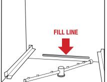
Hold down "FILL" Switch for approximately 10 - 15 seconds to allow water to flow into the dishwasher. Water should reach "FILL LINE" which is located inside at the back of the wash tank. Close door, then press "START" switch.
