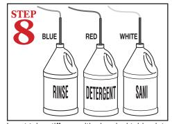
Insert tube stiffener with chemical tubing into corresponding chemical dispensers.
