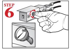
Adjust heater thermostat to 140F.
