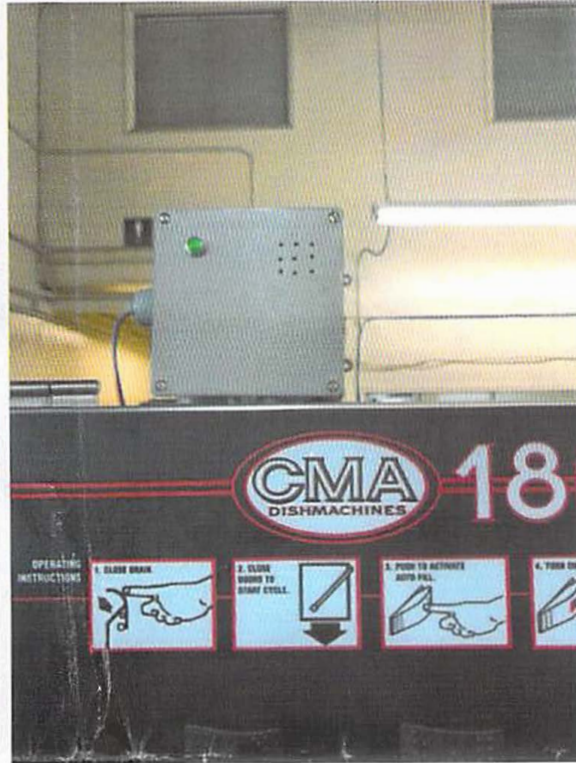
Chemical alarm front view
