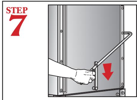
To start machine close the doors. The machine will automatically start and run through its cycle.
