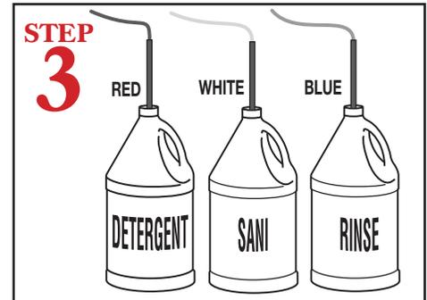
Insert tube stiffener with chemical tubing into each corresponding chemical dispensers.
