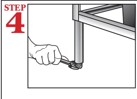
Level dishmachine by adjusting leveling legs. Dishmachine must be level front to back, side to side to ensure proper performance.
