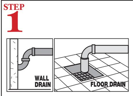
Connect the drain pipe from scrap accumulator to floor or wall drain.
