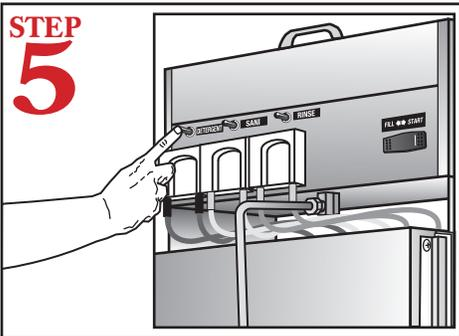
Press and hold down the three Primer Toggle Switches for the chemical pumps until product is discharging into the machine.
