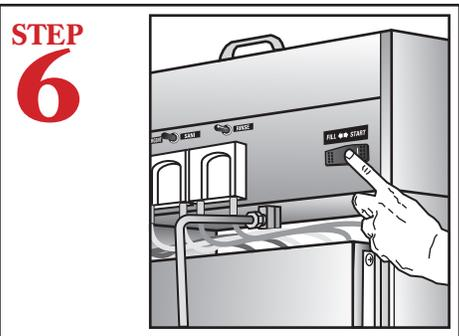
Press and hold the Fill/Start Switch until the water level is approximately 1/2" to 3/4" below the overflow hole in the PVC standpipe.
