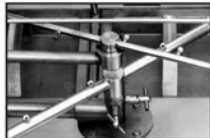
Unique pull-pin design allows wash arms to be easily removed for cleaning.
