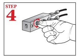
If necessary adjust the temperature by turning the adjustment stem clockwise to increase.
