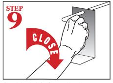
Close drain valve before filling machine with water.
