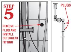
Remove plug to install detergent fitting. Remove plugs from the mixing chamber to install sani/rinse injection fitting (sanitizer, detergent and rinse injection fittings provided by dispenser manufacturer, CMA does not supply.)
