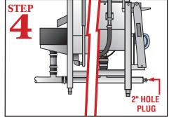
Connect drain at either end of the horizontal drain pipe from wash tank or scrap trap drain.
