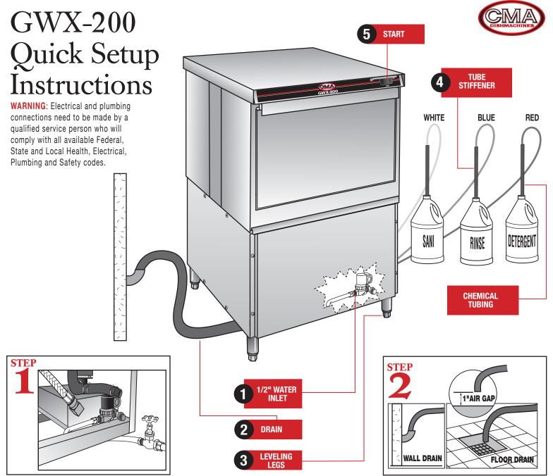
Connect dishmachine to hot water source, recommended 140° (120° minimum temperature required) using a 1/2" connector.
